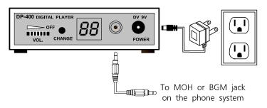
Connect the power supply and the audio patch cord. Two different audio patch cords are provided. Use the one that fits your phone system.
